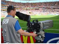
With the capability of recording up to 300 fps, the Hi-Motion is ideal for slow-motion playback for broadcast sporting events.
